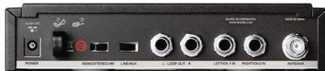
Back panel I/O facilities on the P3T transmitter.
