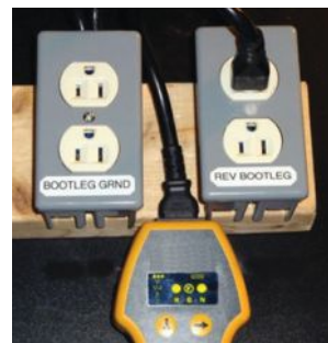
Figure 4: A ground impedance tester can identify a receptacle with a bootleg ground, but it can’t tell if the outlet has correct or reverse polarity.
