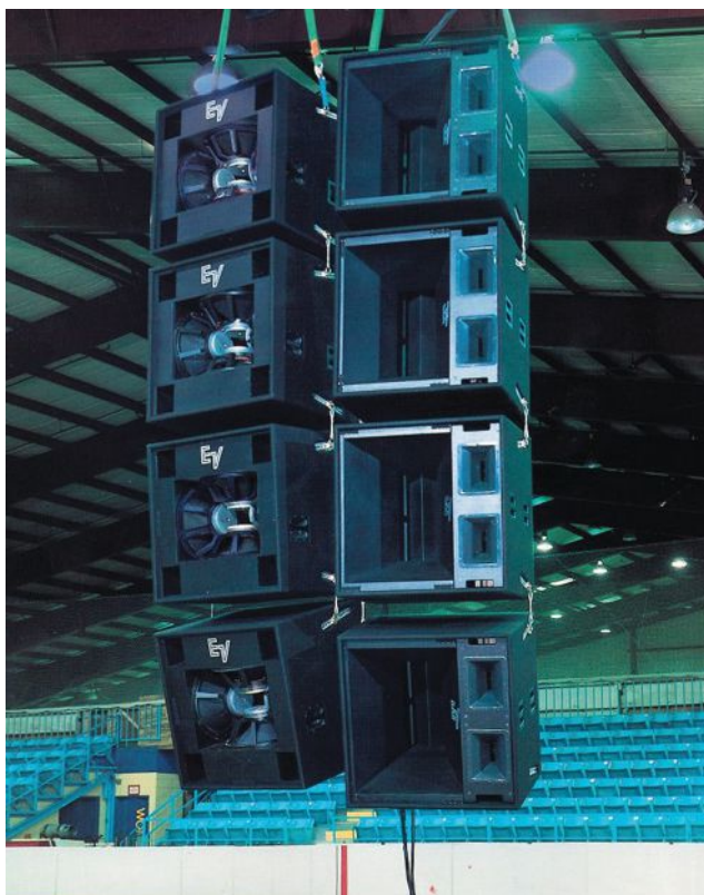
Iconic Electro-Voice MTL-4 subs (each with four 18-inch woofers), a staple of the touring circuit in the early to mid 1990s, flying with their mid/high companions.
