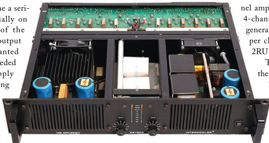
The 2-channel Lab.gruppen SS 1300 with Intercooler technology.
