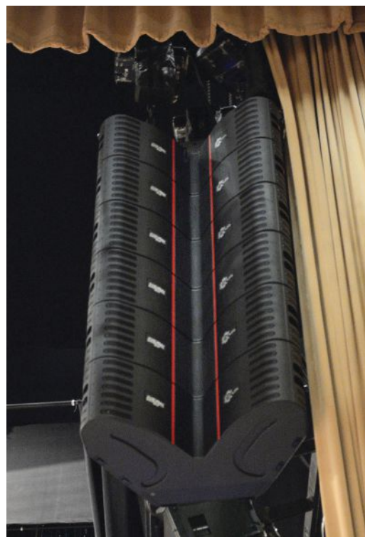
Above, system tech Andrew Dowling (left) and front of house engineer Gary Lewis at the Midas XL4 analog console during a show. Below, a look at one of the six-module EAW Anya arrays deployed at a theatre.
