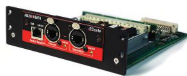
The M-DL-ADAPT interface fits in any dLive I/O port and adds compatibility with most iLive/GLD networking cards, including Dante, Waves, ACE, MADI and more.
