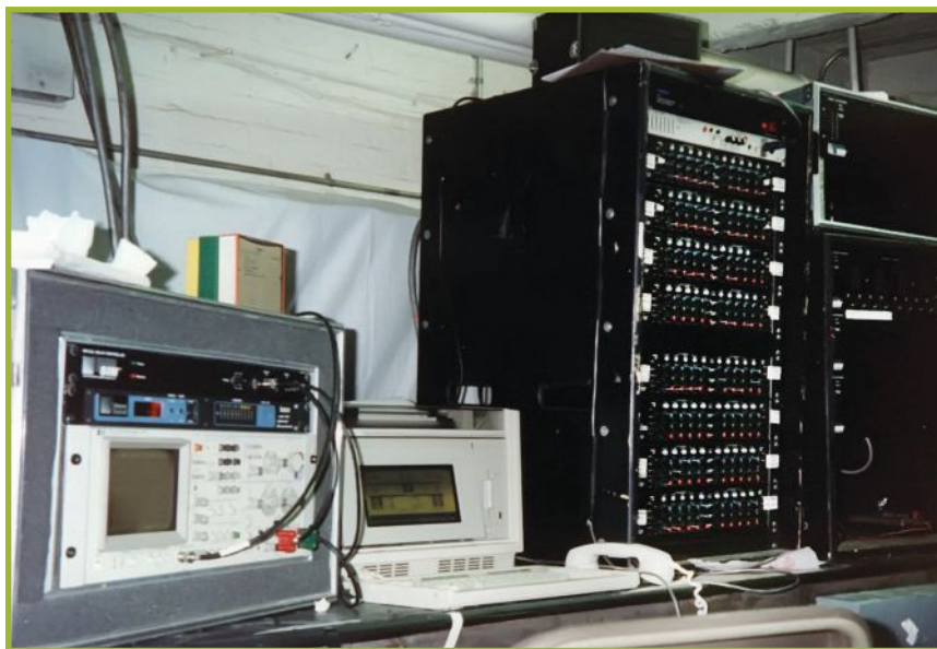
SIM in action for Les Miserables in Boston (1988 or 89). Notice that the analysis system is larger than the signal processing (EQs and delays) that it's monitoring.
