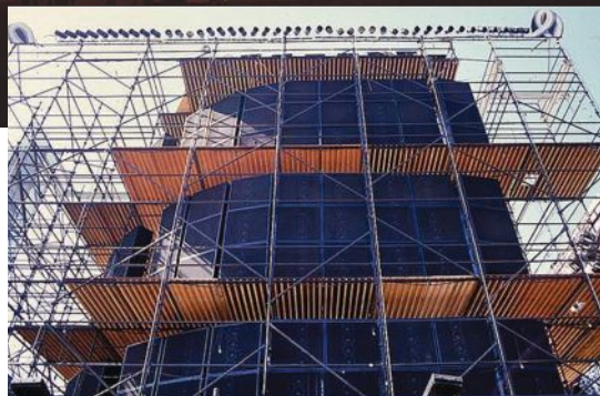
Figure 5: A closer look at the modular Clair S4, each loudspeaker housing 10 JBL transducer components.
