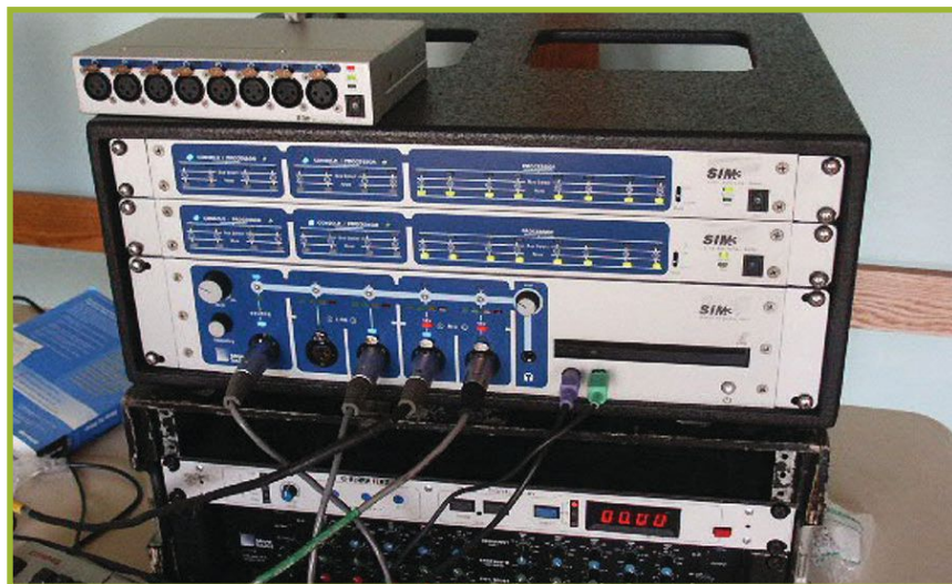
SIM 3 (2003) represented an incremental expansion of capability, ease of operation and reduction of size, helping the optimization process become more mainstream.
