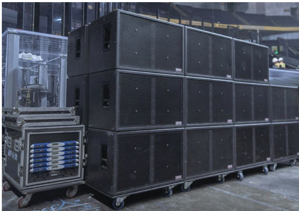
Above, Adam Levine making his way out on the stage thrust with Shure UHF-R transmitter in hand on the current tour. Above right, The SB2001 subwoofer configuration, with Powersoft K Series amplifiers rack-mounted alongside. Below right, System tech Andrew Dowling (left) and house engineer Jim Ebdon at front of house.
