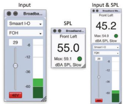
Figure 4: Further metering capabilities.
