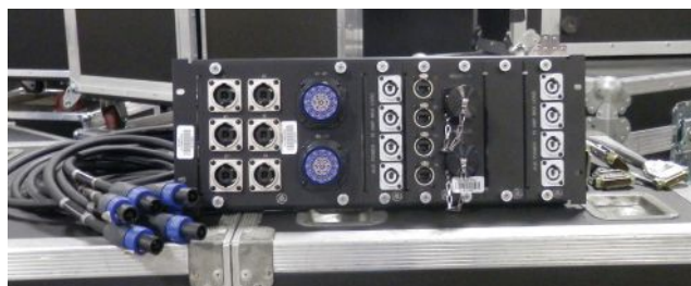
A prototype of the panel with a Socopex module designed for a d&b systems.
