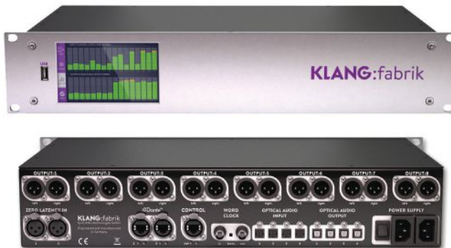
The KLANG:fabrik Dante-enabled digital processor that’s at the heart of the system.
