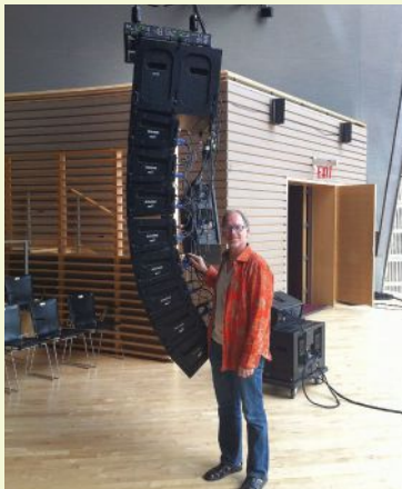
A modern era line array system (and the author) at the Appel Room, Jazz at Lincoln Center in New York. The main system is subdivided into four channels of signal processing (sub +3), and the various fill systems have independent processing as well.
