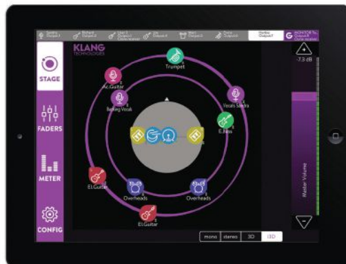
KLANG:app GUI allows remote control of 3D panning.
