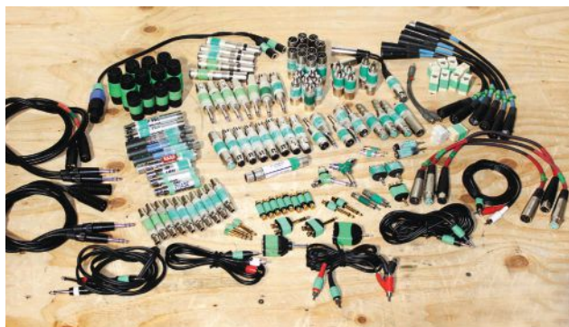
Barrels and cable adapters that the author carries to shows and events. There are dozens more of each type in his company workboxes. Note the green ID tape to help prevent these items from "growing legs."
