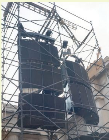
The main system shown here for the Grateful Dead at the Greek Theater in Berkeley (1984) had minimal subdivision, entirely driven by a single channel of equalization with no delays or relative level adjustment. The standard optimization options of a modern system (macro and micro delay, relative gain adjustment and separate EQ for the uppers/lowers/side fills/etc. were not available options at that time.
