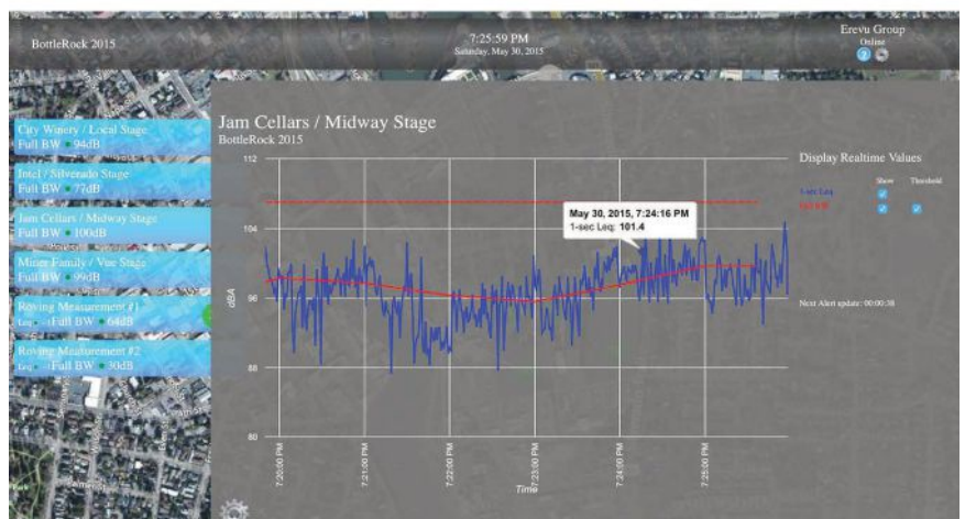
Screenshots of the Leq and other information measured over time at multiple stages at BottleRock 2015. While the Miner Family Winery Stage faced south toward the Napa River, two of the other main stages faced residential and commercial areas. Both showed significant improvement with regard to noise mitigation, despite Erevu moving its measurement locations outside the grounds 1,000 feet closer to both stages.
