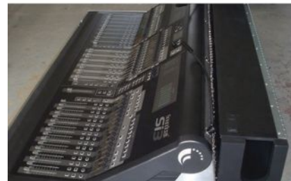
It's important to ensure that doghouses have enough room for cabling. They can also serve as a handy shelf when closed.
