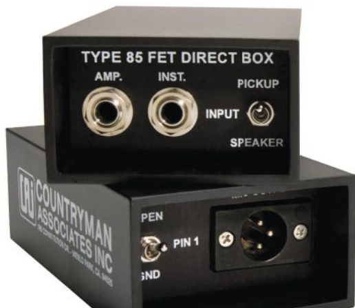
The Countryman Type 85 active direct box exhibits a polarity that's opposite of modern DIs.
