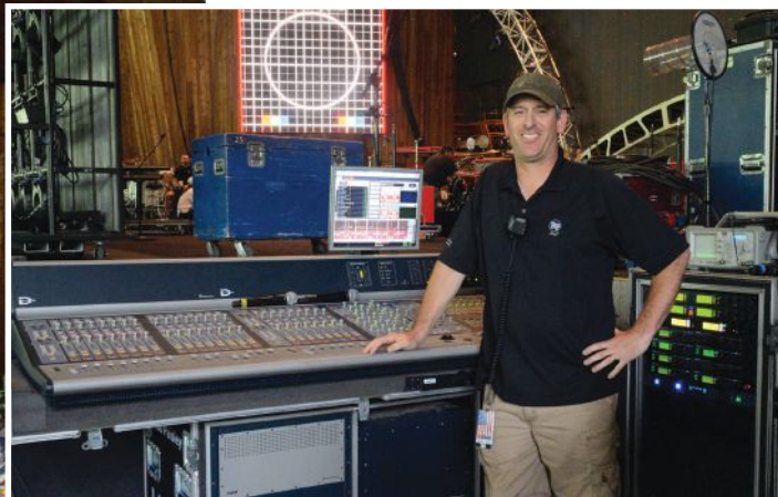
Monitor engineer Mark Gould with his Avid D-Show, and immediately behind him are the tour's Shure UHF-R wireless receivers topped by the Madell RF spectrum analyzer that he uses for frequency coordination.
