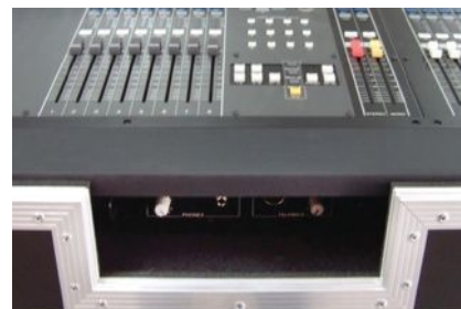
Trays can also be modified to accommodate additional gear like outboard talkback mic interface and headphone jack.
