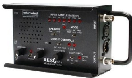
Figure 7: A specialty tester for AESx interfaces. COURTESY WHIRLWIND
