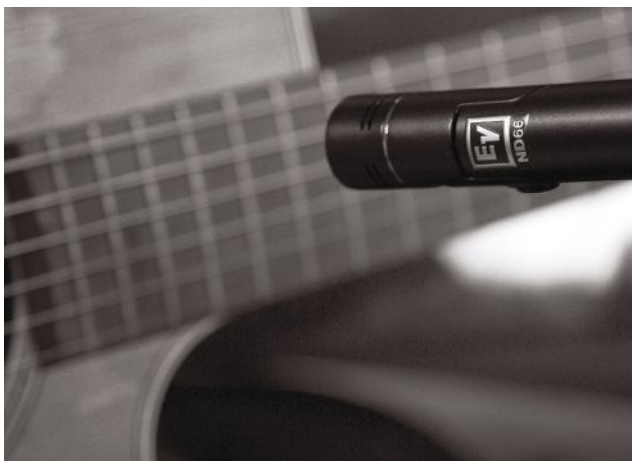
An Electro-Voice ND66 small-diaphragm condenser capturing an acoustic guitar.
