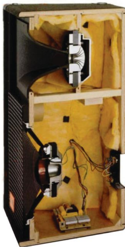
A nifty cutaway view of a JBL SR Series II loudspeaker (circa 1997) that shows the placement of the cone and compression drivers.
