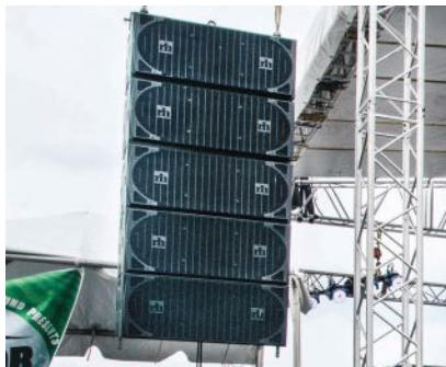
A main array comprised of Renkus-Heinz STXLA/9 cabinets.
