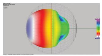
Figure 2: Horizontal directivity balloon of a 12-inch 2-way loudspeaker at 500 Hz (box facing left).
