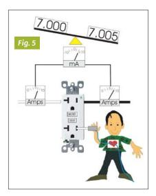
stays activated. If the current flow is unmatched by any more than 5 mA, say by someone touching a live wire and the earth at the same time, then the trigger circuit inside trips a little switch and the current flow is stopped. It's that simple.
