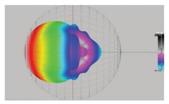
Figure 3: Horizontal directivity balloon of a 12-inch, 2-way loudspeaker at 800 Hz (box facing left).
