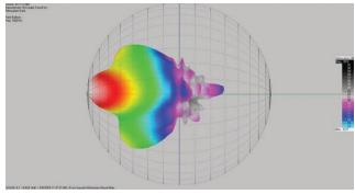
Figure 5: Vertical directivity balloon of a 12-inch, 2-way loudspeaker at 1,600 Hz, crossover at 1,350 Hz (box facing left).
