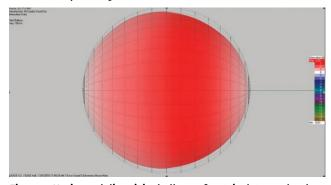
Figure 1: Horizontal directivity balloon of a 12-inch 2-way loudspeaker at 100 Hz (box facing left).
