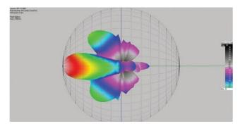
Figure 4: Vertical directivity balloon of a 12-inch, 2-way loudspeaker at 1,250,Hz, crossover at 1,350 Hz (box facing left).
